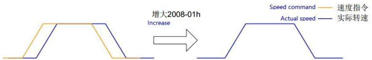
Figure 7-1 Velocity loop gain
