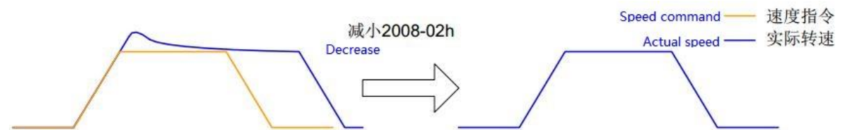
Figure 7-2 Velocity loop integration time constant
