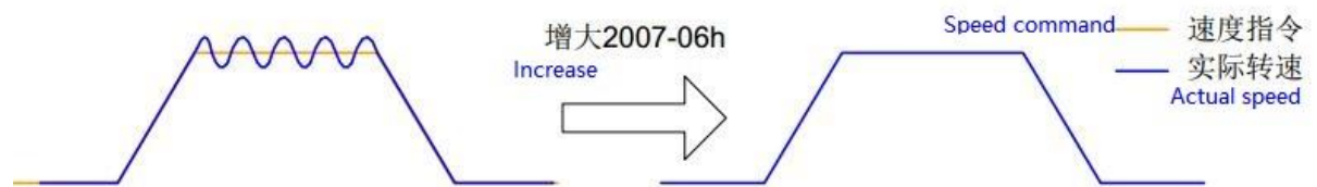
Figure 7-4 Torque command filtering time constant
