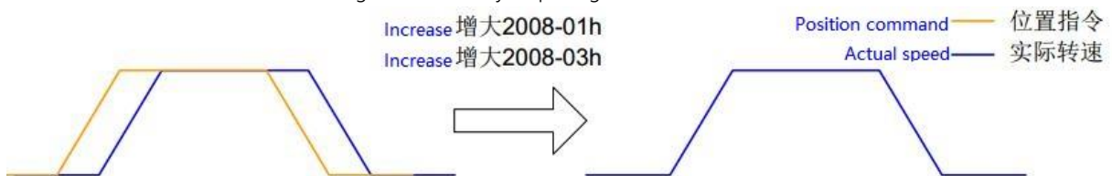
Figure 7-3 Position loop gain
