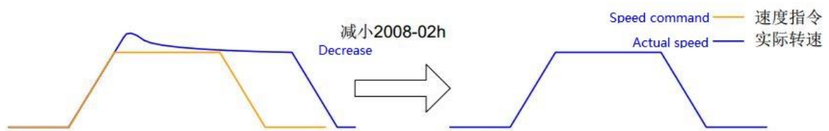
Figure 7-2 Velocity loop integration time constant
