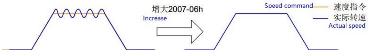
Figure 7-4 Torque command filtering time constant
