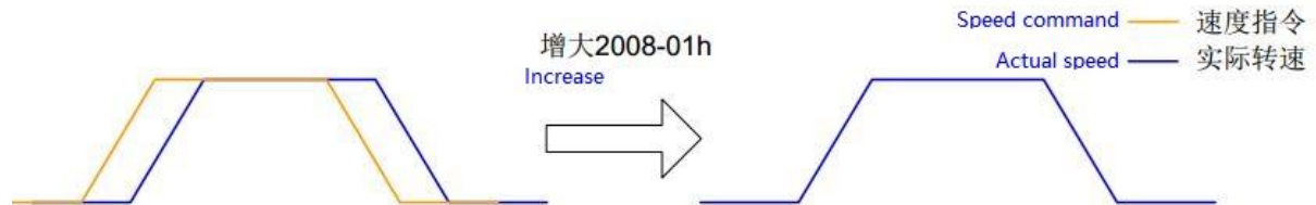
Figure 7-1 Velocity loop gain
