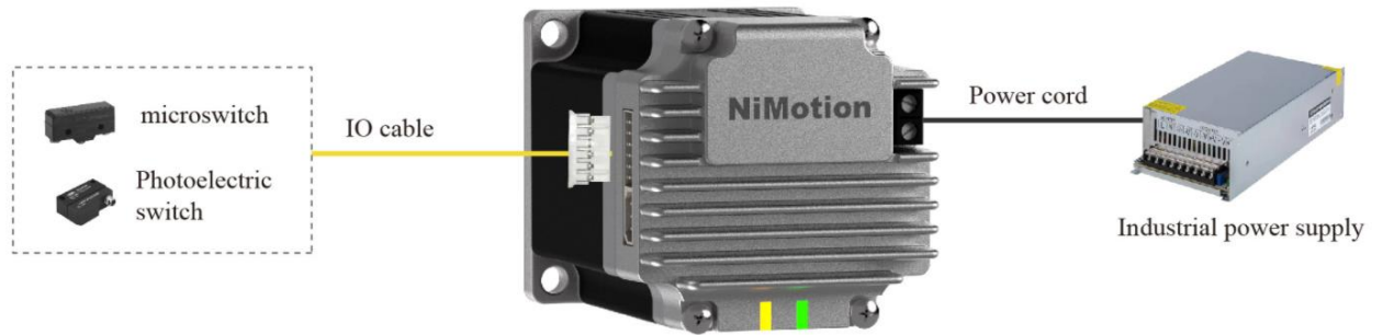
Figure 3-6 External Control Wiring Diagram
